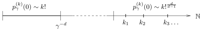
Figure 4: The derivatives of the pressure at h = 0 , when \gamma > 0 . The first ones ( k \leq \gamma^{-d} ) behave like those of an analytic function, but non-analyticity always dominates for large k .
